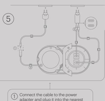
adapter and plug it into the nearest power socket. Connect the two USB-C cables to the
